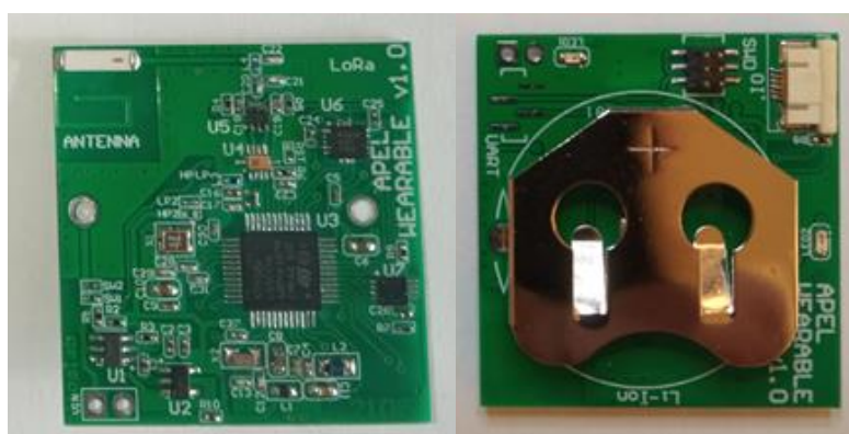
Figure 2. Printed Circuit Board of the wearable device - version 2
