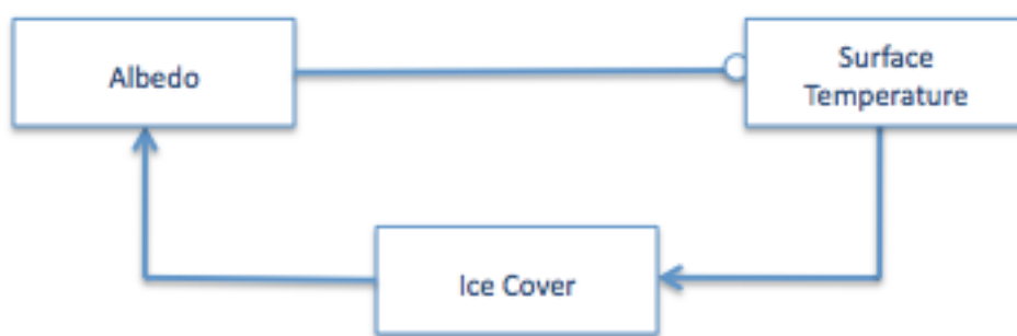
Figure 3 - An example of a positive feedback loop, where an increase in albedo results in a reduction in surface temperature, allowing ice cover to increase which, in turn, further increases albedo.
